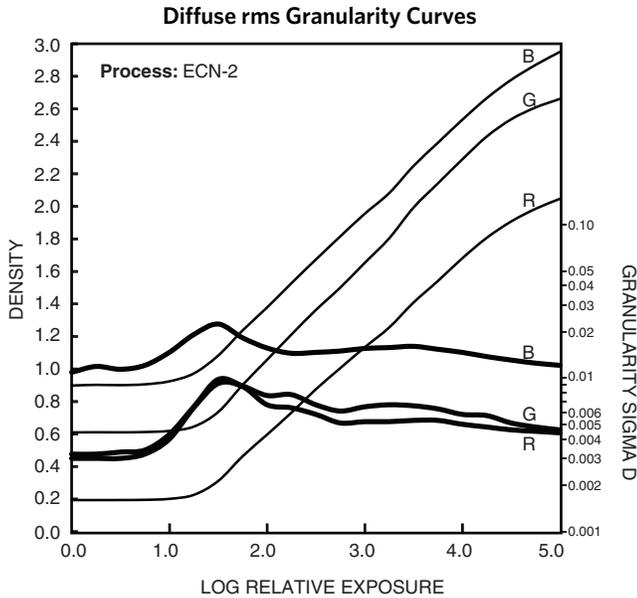
To find the rms Granularity value for a given density, find the density on the left vertical scale and follow horizontally to the characteristic curve and then go vertically (up or down) to the granularity curve. At that point, follow horizontally to the Granularity Sigma D scale on the right. Read the number and multiply by 1000 for the rms value.
