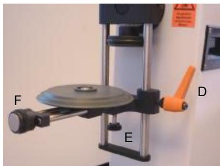
Fig. 4 Adjustment of the lower tank holder
